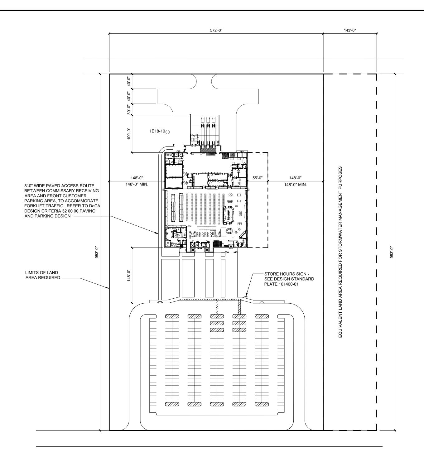
1E18-10 8'-0" WIDE PAVED ACCESS ROUTE BETWEEN COMMISSARY RECEIVING 122'-0" 126'-0" AREA AND FRONT CUSTOMER 82'-0" MIN. 82'-0" MIN. PARKING AREA, TO ACCOMMODATE FORKLIFT TRAFFIC. REFER TO DeCA DESIGN CRITERIA 32 00 00 PAVING AND PARKING DESIGN — SEE DESIGN STANDARD PLATE 101400-01 LIMITS OF LAND AREA REQUIRED -
